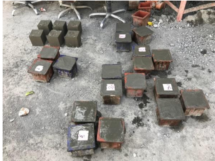
Fig 5 : Concrete Cubes for compression testing.
