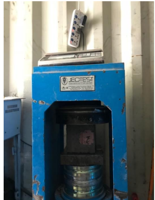
Fig 6 : The used lab compression test machine.
