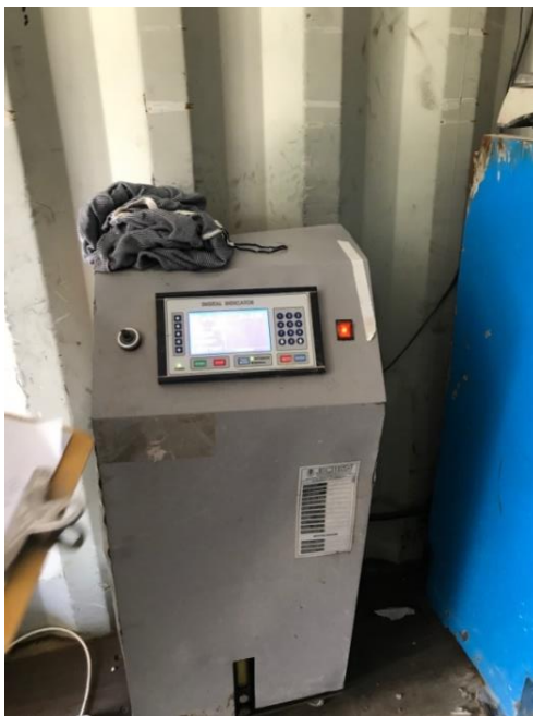
Fig 6 : The used lab compression test machine.
